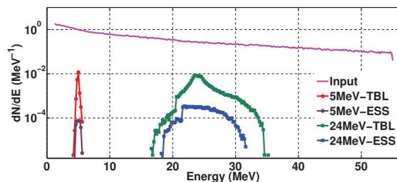
Figure 5: Input and output energy spectra, obtained when only the ESS or the whole transport beamline (TBL) have been simulated.
