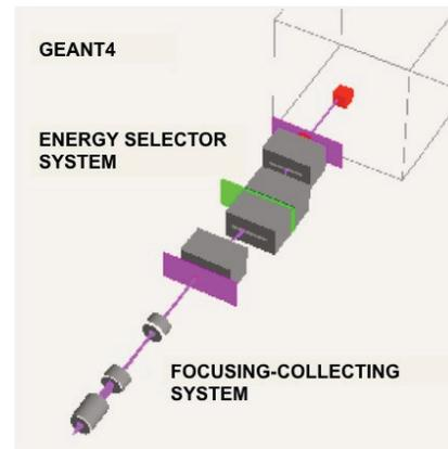
Figure 3: The transport beamline for laser-driven charged particles of the hadrontherapy advanced example of the GEANT4 toolkit.
