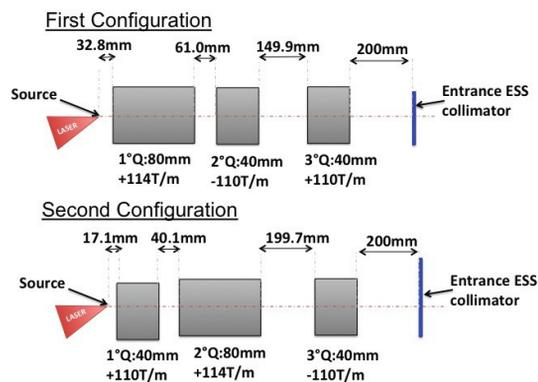
Figure 4: Details of the final PMQs setups, optimized for a 5 MeV (top) and 24 MeV (bottom) proton beam transmission.
