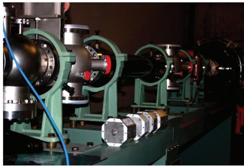
Figure 1: The four quadrupoles at INFN-LNS.
