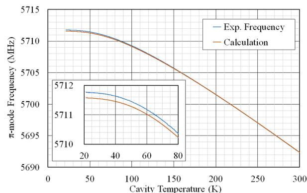
Figure 4: Comparison of temperature dependence of the resonant frequency between the experimental result and the calculated result based on the linear expansion coefficients of OFHC copper from NIST [5].
