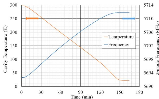
Figure 3: The cavity temperature and the  $\pi$ -mode frequency as a function of the time elapsed since the refrigerator was switched on.
