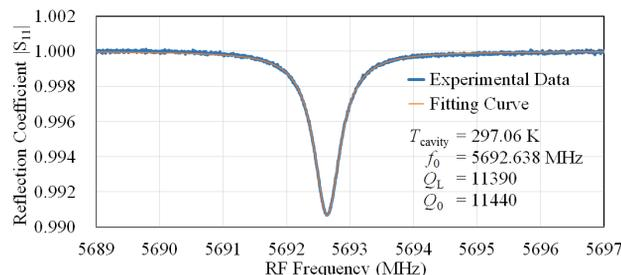
Figure 5: Plot of  $|S_{11}|$  around the  $\pi$ -mode resonance peak at room temperature.
