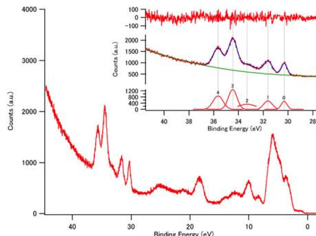
Figure 7: Multi-alkali UPS spectrum as a function of binding energy.
