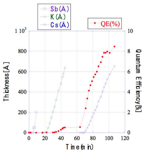
Figure 2: Time course of QE and evaporation thicknesses.
