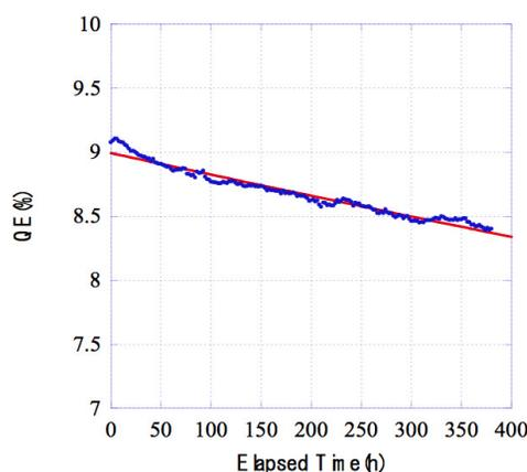
Figure 3: QE degradation as a function of time with blue laser at continuously irradiated area.
