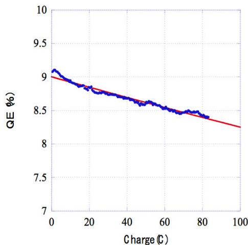
Figure 4: QE degradation as a function of extracted charge with blue laser at continuously irradiated area.
