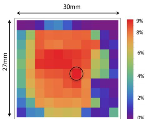
Figure 5: QE map with blue laser on the substrate.
