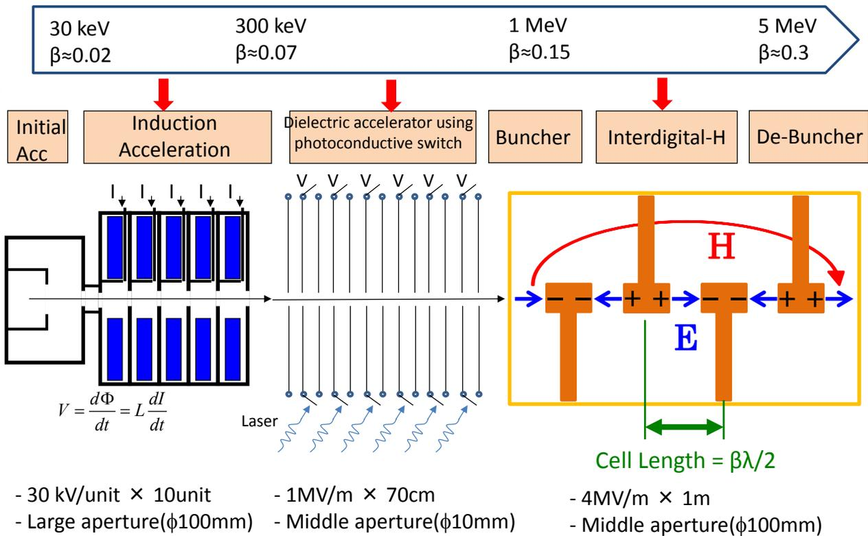
Figure 3: Accelerating system for the re-acceleration at U-line for the muon microscopy.
