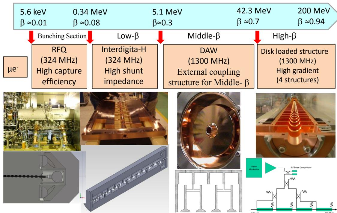
Figure 2: Accelerating system for re-acceleration at H-line for the g-2 experiment.
