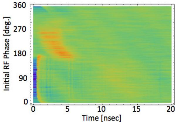
Figure 8: The contour plot of current signals for various RF phases. Positive current were detected in the red area, negative current in the blue, while green indicates no signal.
