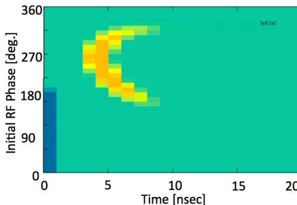
Figure 9: The simulation result of current signal for various RF phase. Positive/negative current is indicated as red/blue, and green indicates neutral.
