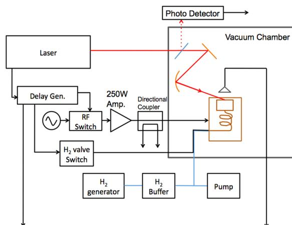
Figure 2: Image of Experimental Layout.
