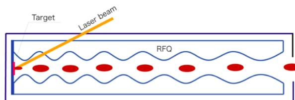
Figure 1: Schematic image of RFQ with initially-bunched ion beams.
