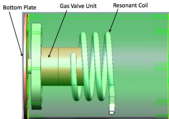
Figure 4: A internal view of the RF resonator.
