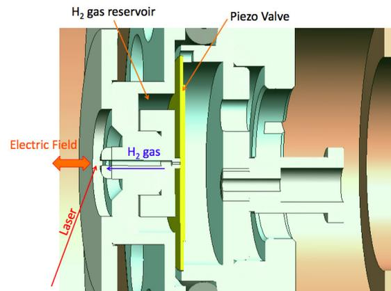
Figure 5: Cross sectional view of the gas valve unit in the resonator.
