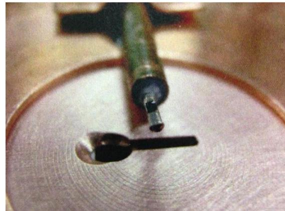
Figure 6: Ion probe made by cutting and stripping a semi-rigid coaxial cable. The probe was attached on the bottom plate of the resonator.
