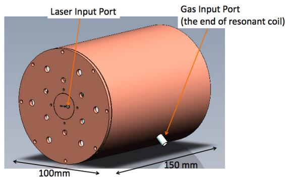
Figure 3: An entire view of the RF resonator.
