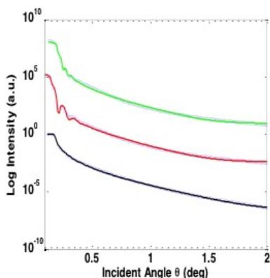
Figure 3: Sample 3: XRR measurements (open circles) and data simulation (colored lines) of a co-deposition cathode. The fit for the Si substrate (black), the K-Sb phase (red) and the Cs-K-Sb phase (green). For this cathode K and Sb were first co-deposited, followed by Cs-Sb co-deposition, similar to the growth mode described by [5]
