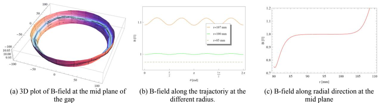
Figure 4: B-field distribution of 360° Bending Magnet (All are calculated curves and graph using fitting equation).
