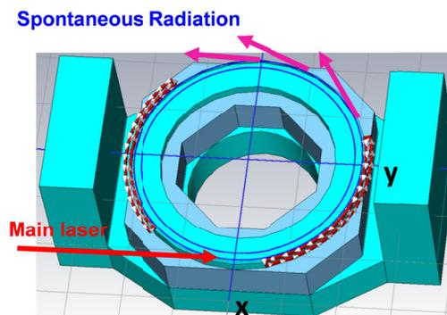
Figure 3: Schematic of 360° Bending Magnet
