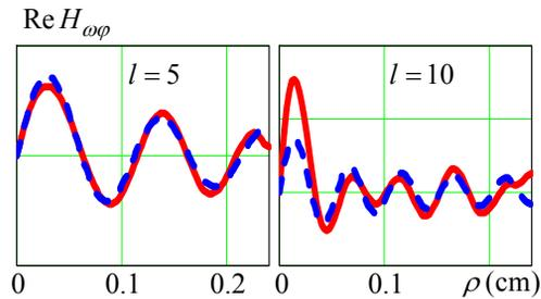
Figure 2: The behaviour of  $H_{\omega\phi}$  component over the waveguide aperture  $\rho < a$ ,  $z = +0$ . Solid (red) line is calculated using solution of (17), dashed (blue) line is calculated using approximate technique from [2]. Mode frequency is  $\omega_{20} = 2\pi \cdot 412$  GHz,  $a = 0.24$  cm,  $\varepsilon = 10$ ,  $\gamma = 7$ . Waveguide supports 21 propagating modes.
