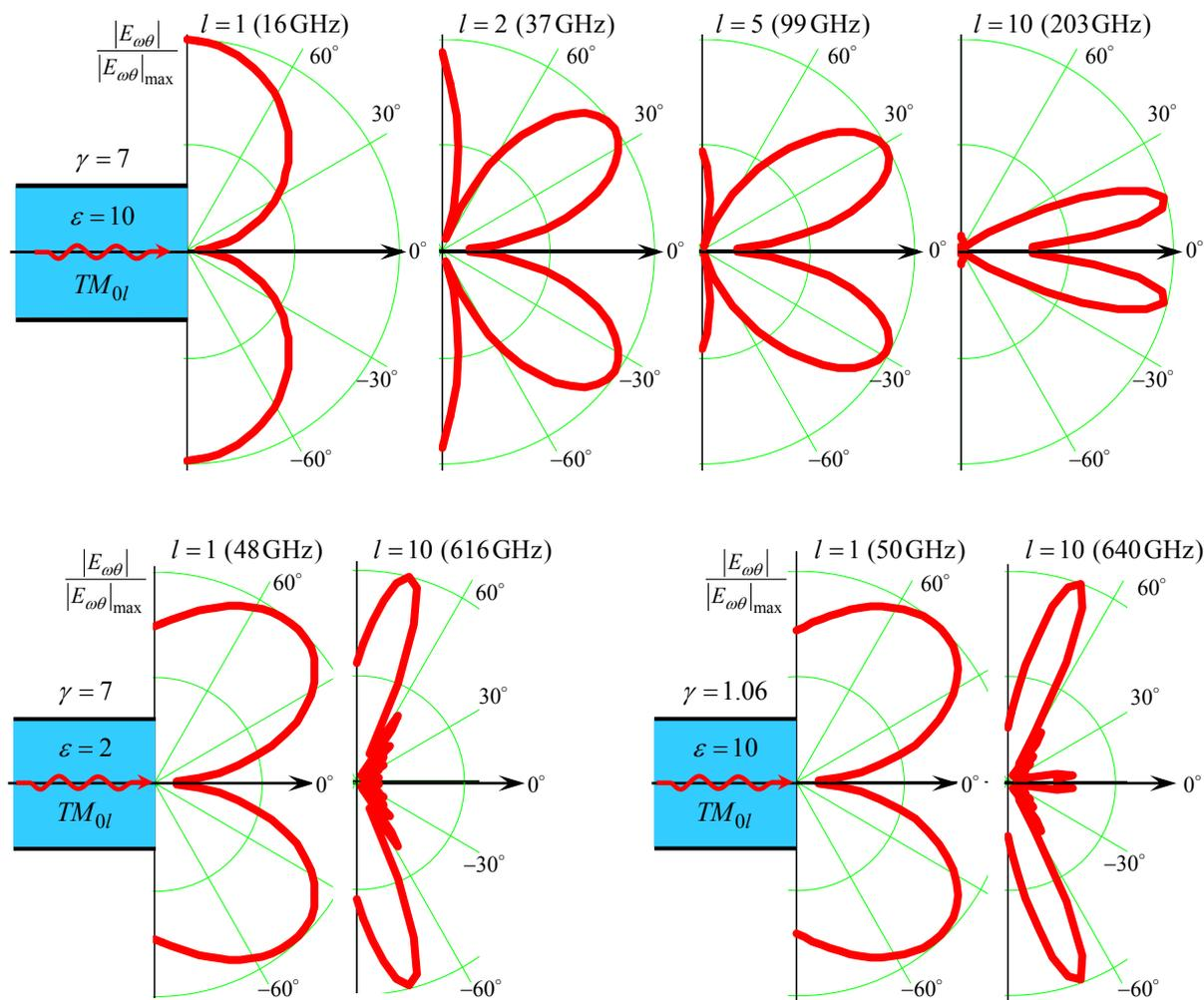
Figure 3: Radiation patterns (normalized  $|E_{\omega\theta}|$  versus  $\theta$ ) in the Fraunhofer zone (21) produced by  $TM_{0l}$  mode at the open end of dielectrically loaded waveguide with  $a = 0.24$  cm. Frequency  $\omega$  (shown near each pattern) is chosen to be equal to the frequency of  $l$ -th mode of Cherenkov radiation (20) produced by the charge with Lorentz factor  $\gamma$ .
