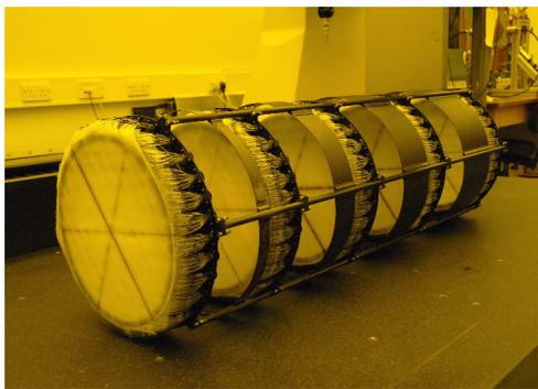
Figure 3: Photograph of one of the MICE Trackers, showing the 5 stations and the 3 doublet planes of scintillating fibres at  $120^\circ$  angles.
