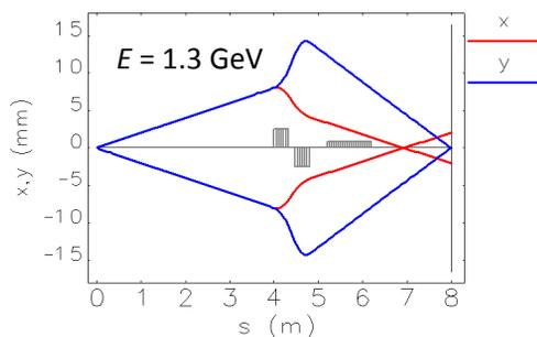
Figure 4: ELEGANT [11] simulation results showing the trajectories of electrons with angles at the plasma cell of  $\pm 2$  mrad. The first quadrupole has  $K_1 = +4.07 \text{ m}^{-2}$  and the second quadrupole has  $K_1 = -4.07 \text{ m}^{-2}$ .
