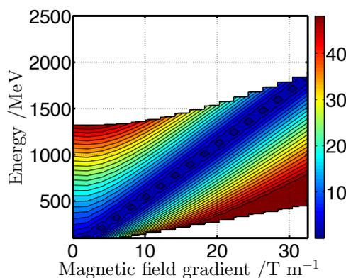
Figure 5:  $\Delta E/E$  as a function of energy and quadrupole strength with the HB4 dipole current at 40A for the "negative" beam.
