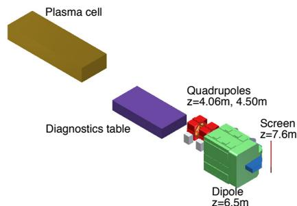
Figure 1: A 3D CAD image of the spectrometer system annotated with distances along the  $z$  direction from the exit of the plasma cell to the magnetic centres of magnets, and the centre of the scintillator screen.
