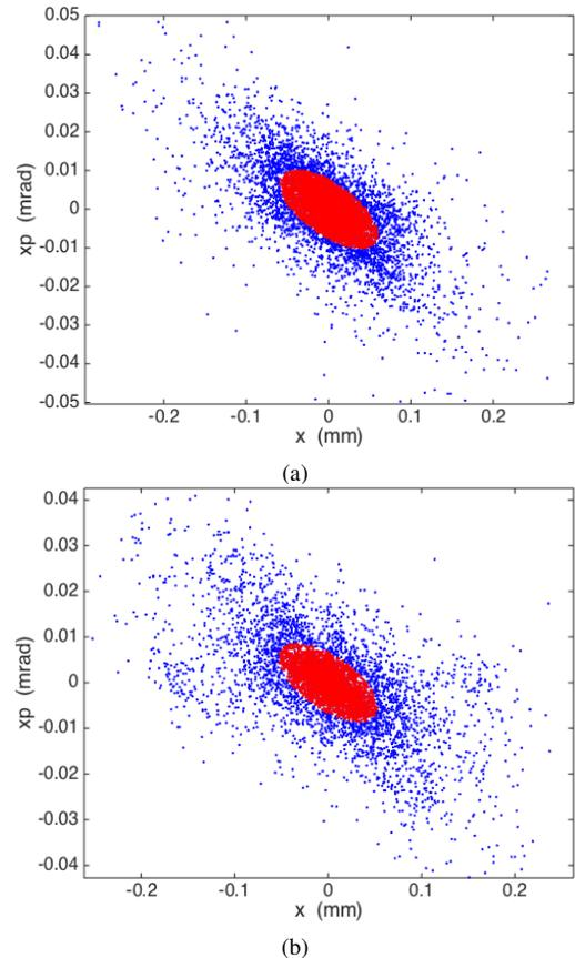
Figure 4: Reconstructed phase spaces at (a)  $100 \text{ m}$  and (b)  $500 \text{ m}$  during the beam passage through a Li gas column. Particles within the  $1\sigma$  of the Courant-Snyder ellipses are shown in red.
