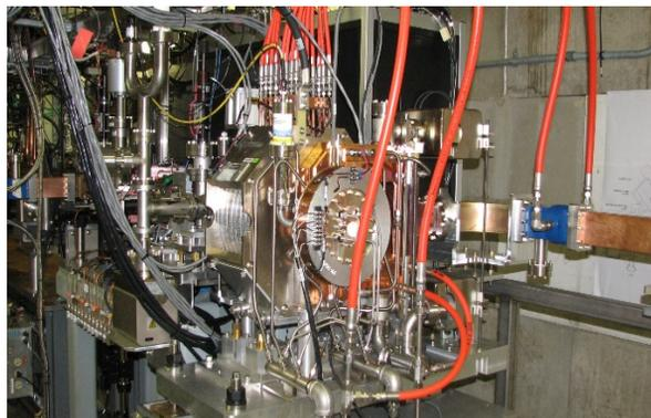
Figure 1: PC Gun Installed in the APS Linac Tunnel.
