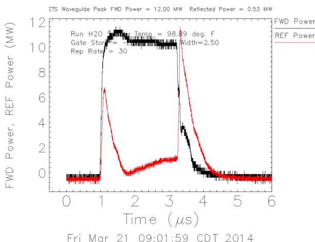
Figure 4: Forward and Reflected RF Waveforms. (Measured at PC Gun Waveguide).
