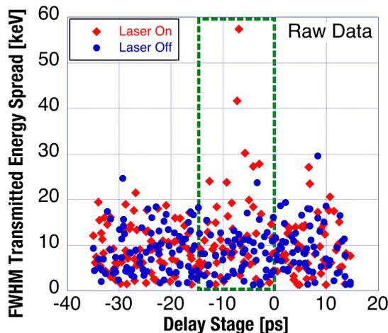
Figure 2: Time correlation data, showing energy spread of the transmitted electron population versus relative laser-electron timing. Energy modulation is observed near  $-7$  ps for laser-on shots (red) but not laser-off (blue).
