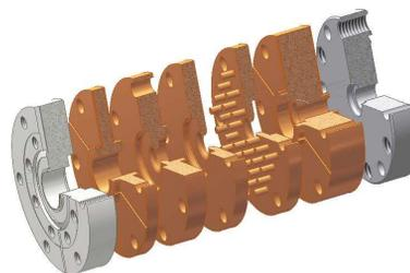
Figure 1: Expanded three quarter section view of the solid model of the 17 GHz PBG structure, showing two coupling cells and central PBG cell. Power is coupled in from the left.
