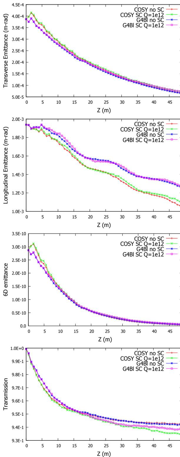
Figure 3: In order from the top, the transverse, longitudinal, 6D emittance, and transmission behavior with and without space charge through 60 cells as simulated in both codes.
