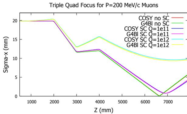
Figure 1: This plot compares the simulated deviation in  $x$  of a particle bunch through three quadrupole magnets tuned to focus the muons to a point. For varying amounts of total charge, COSY and G4Beamline are in good agreement.
