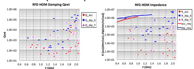
Figure 5: The  $Q_{ext}$  and impedance of the HOMs.
