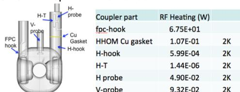
Figure 8: RF heating due to operating mode.
