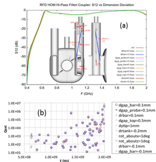
Figure 6. Sensitivity of  $Q_{ext}$  on coupler dimension errors.
