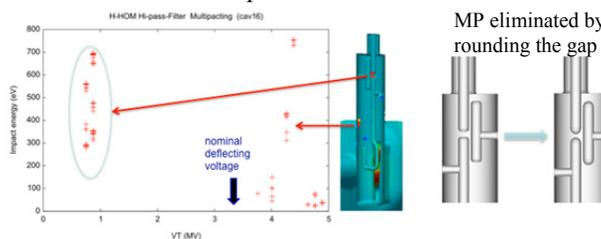
Figure 10: MP band in the high-pass filter HOM coupler. The MP band was eliminated by rounding the gap.
