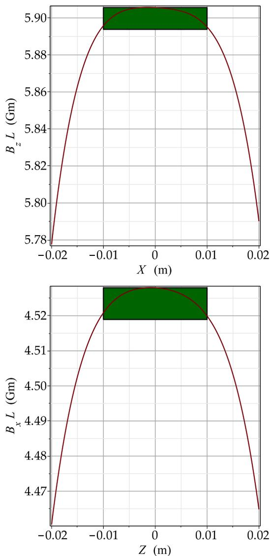
Figure 4: Top frame: Vertical field vs. horizontal coordinate. Bottom frame: Horizontal field vs. vertical coordinate. The box represents  $\pm 0.1\%$  tolerance over  $\pm 1$  cm
