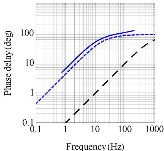
Figure 5: Phase shift vs frequency due to the vacuum chamber. Blue lines are calculations (solid line) and measurements (dashed line) for copper chamber; the black dashed line of the calculation for a stainless steel chamber. Wall thickness is 6 mm in all cases.
