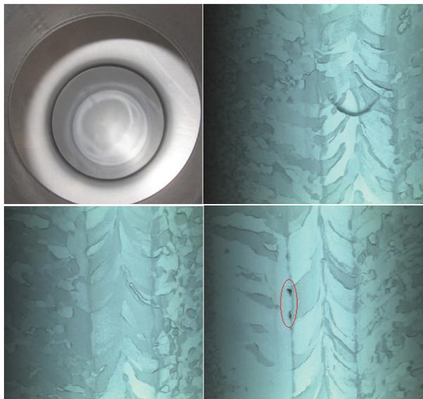
Figure 3: Optical inspection pictures of ALD3. Top left picture shows the coated surface of the cavity looking from one of the beam tubes. Top right and bottom left pictures show characteristic equatorial weld regions of the coated cavity. Bottom right picture shows equatorial region with a couple observed features (marked with the red circle).
