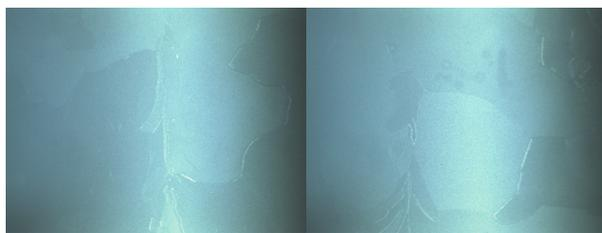
Figure 4: Coated Nb<sub>3</sub>Sn surface as seen with KEK inspection system. The left picture shows characteristic equatorial weld regions of the coated cavity. The right picture shows equatorial region with a couple observed features.
