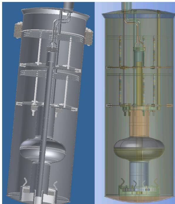
Figure 1: The Nb<sub>3</sub>Sn insert drawing with a 1.3 GHz single cell cavity after(to the left) and before(to the right) conversion to vertical position. Note that Nb cylinder was split at the top with wire EDM to allow for 14" conflat stainless steel flange.
