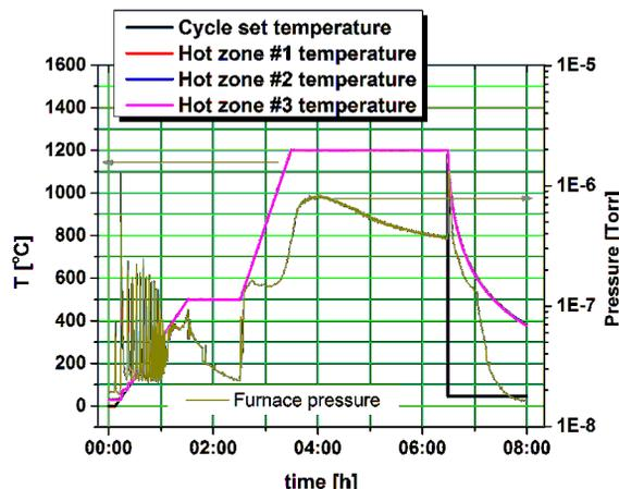
Figure 2: In this plot the temperature and pressure profile from the first Nb<sub>3</sub>Sn cavity coating run are shown. Note the three separate regions: first, the temperature is increased at 6 °C per minute, then, it is parked at 500 °C to allow for SnCl<sub>2</sub> evaporation, then, the temperature is increased at 12 °C per minute to 1200 °C, where the furnace is parked for 3 hours, finally, the heat is turned off and the furnace is cooled down.
