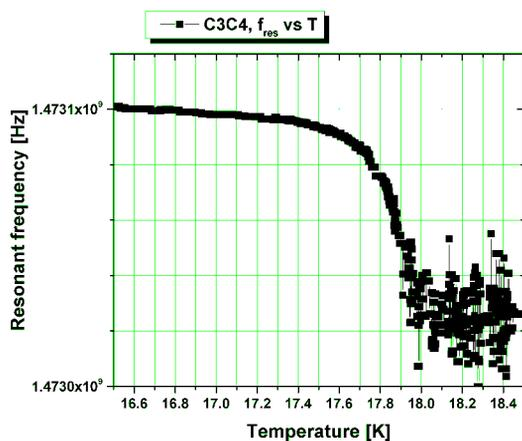
Figure 5: C3C4 resonant frequency vs. average diode temperature. The critical transition temperature is  $17.9 \pm 0.25$  K.
