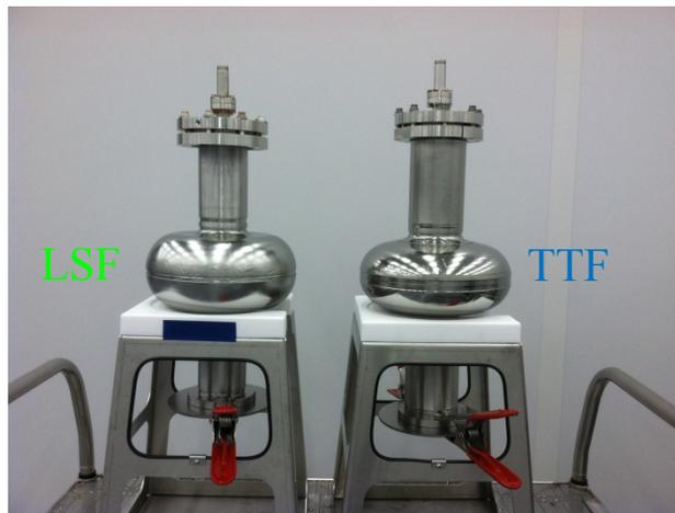
Figure 1: First 1-cell 1.3 GHz LSF shape cavity (L) made of large-grain Nb. A TTF shape 1-cell large-grain Nb cavity (R) is also shown for comparison.
