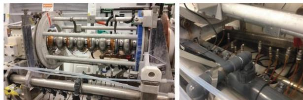
Figure 1: Left: LCLS-II R&D cavity prepared for EP at JLab. Right: Arrangement of water-spray nozzles for external cooling of cavity walls.
