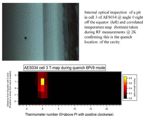
Figure 3: Quenching defect from AES034 doping round 1.
