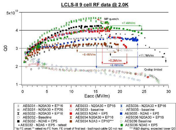
Figure 1: All RF test results for the 6 - 9 cell cavities.
