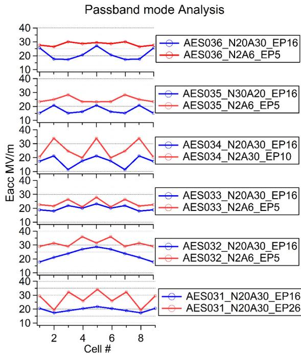
Figure 2: Passband mode analysis for all quench limited tests, separated by cavity for comparison.
