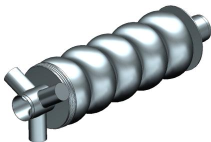
Figure 6: Concept for ERL cooler cavity.
