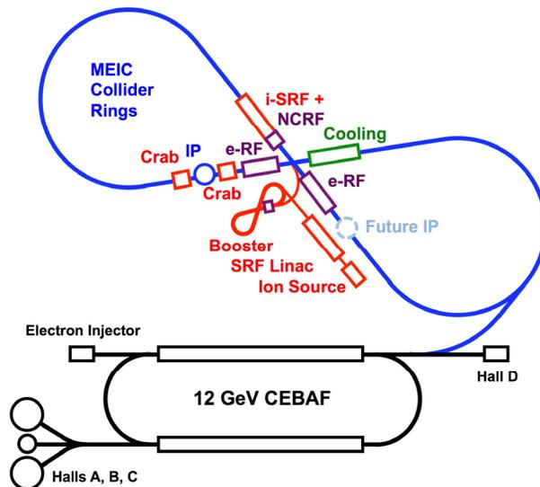
Figure 1: Schematic layout of figure-8 MEIC.
