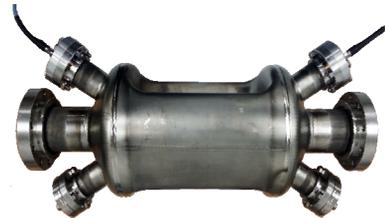
Figure 3: “RF dipole” crab cavity developed by ODU.
