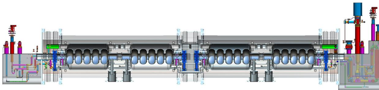
Figure 4: Concept for a versatile modular cryostat to house various MEIC SRF cavities (ERL concept shown).
