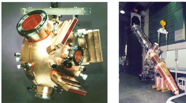
Figure 2: PEP-II RF cavity and 1.2 MW klystron.
