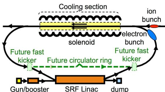
Figure 5: schematic of bunched beam cooler with option for future recirculation.
