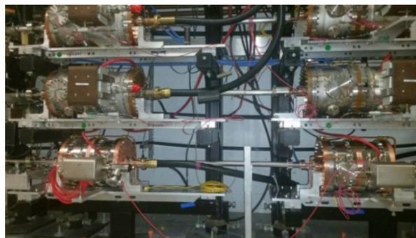
Figure 8: The 1<sup>st</sup> and 2<sup>nd</sup> 750 MHz cavities installed on the 5<sup>th</sup> beam pass of CEBAF under the 500 MHz cavities.
