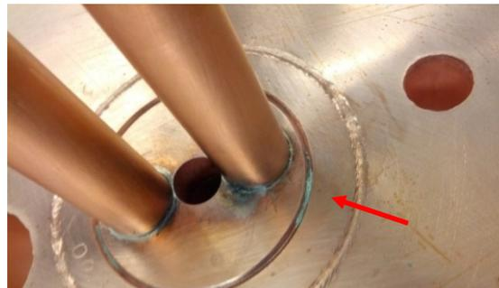
Figure 7: Chemical residual left on the prototype cavity caused a MP barrier and electron activity in its high power test.
