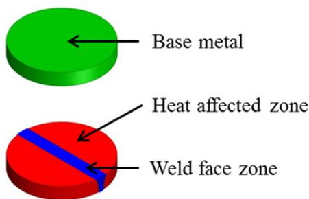
Figure 4: Sketches of the two types of samples.
