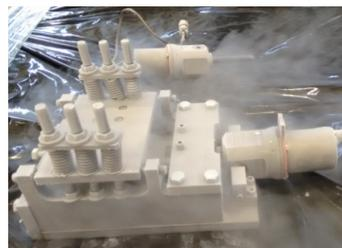
Figure 2: Tuner test stand after liquid nitrogen testing.
