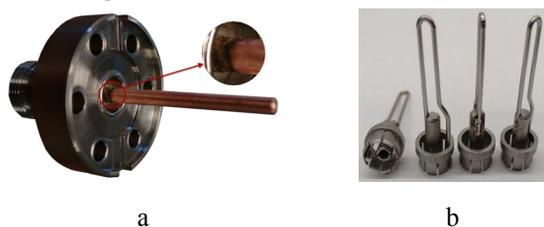
Figure 5: a. 3-cell main coupler after electrical breakdown; b. 3-cell measure coupler loops.
