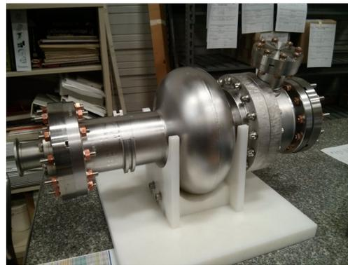
Figure 4: The quarter-wave coaxial coupler with a single cell cavity.
