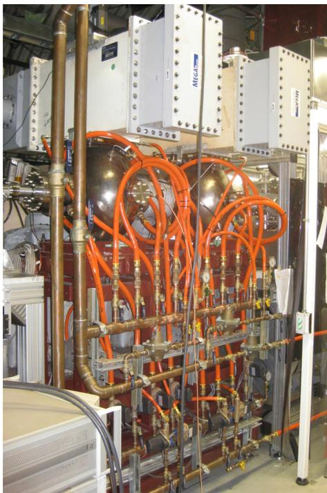
Figure 5: Two bunching cavities in the RHIC tunnel.
