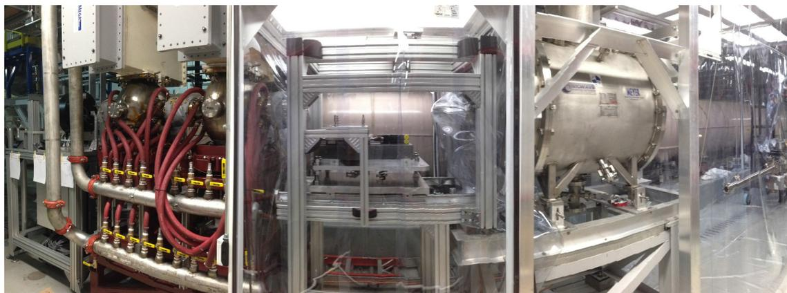
Figure 2: The 112 MHz SRF gun and two bunching cavities in the RHIC tunnel.
