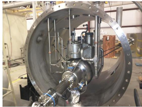
Figure 9: Piping system and He vessel installation.
