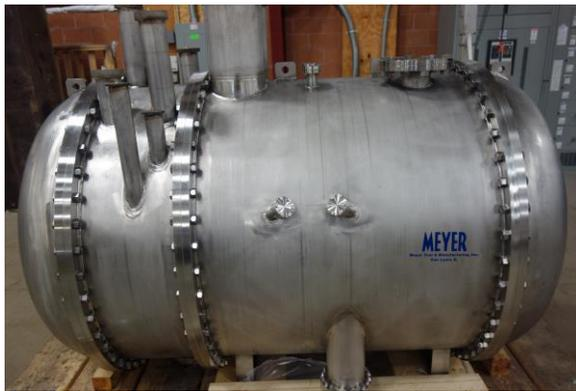
Figure 7: ASME Code stamped vessel.
