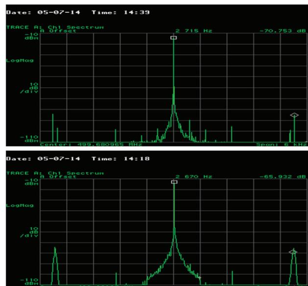
Figure 3: Top: The synchrotron oscillation peak 2.715kHz is clean when away from two times the switching harmonic 2.65kHz; Bottom: The synchrotron oscillation peak 2.67kHz is widened due to beam instability. Large beam horizontal oscillation is observed with a BPM.
