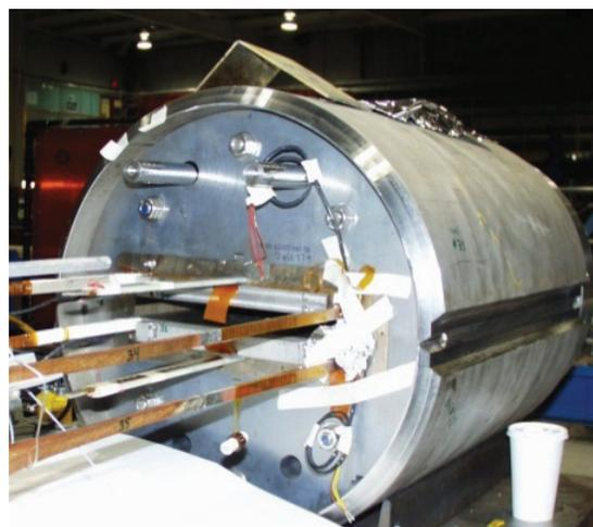
Figure 4: 10 T Nb<sub>3</sub>Sn common coil dipole DCC017 with a large open space for testing insert coil(s).
