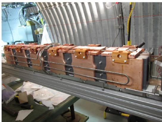
Figure 7: The kicker with Cu cooling plates in the RHIC tunnel.
