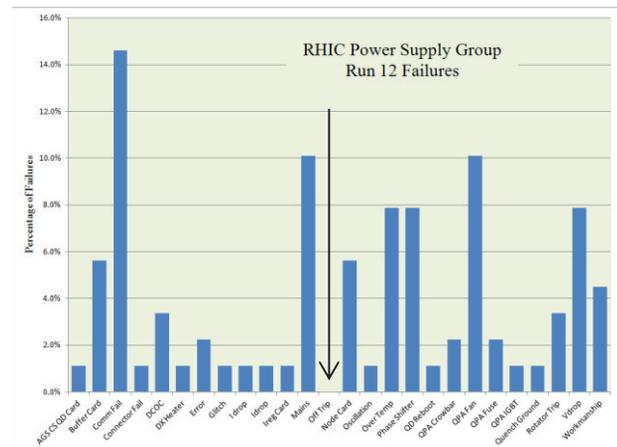
Figure 3: Run 12 Power Supply Failures.
