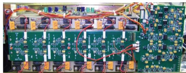
Figure 4: New PCB Installed to Replace Old 3 PCBs in Same Location.
