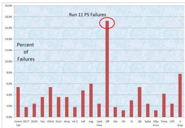
Figure 2: Run 11 Power Supply Failures.
