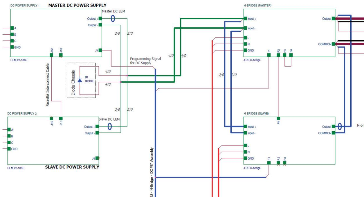
Figure 2: System integration of bipolar qtrim PS system.
