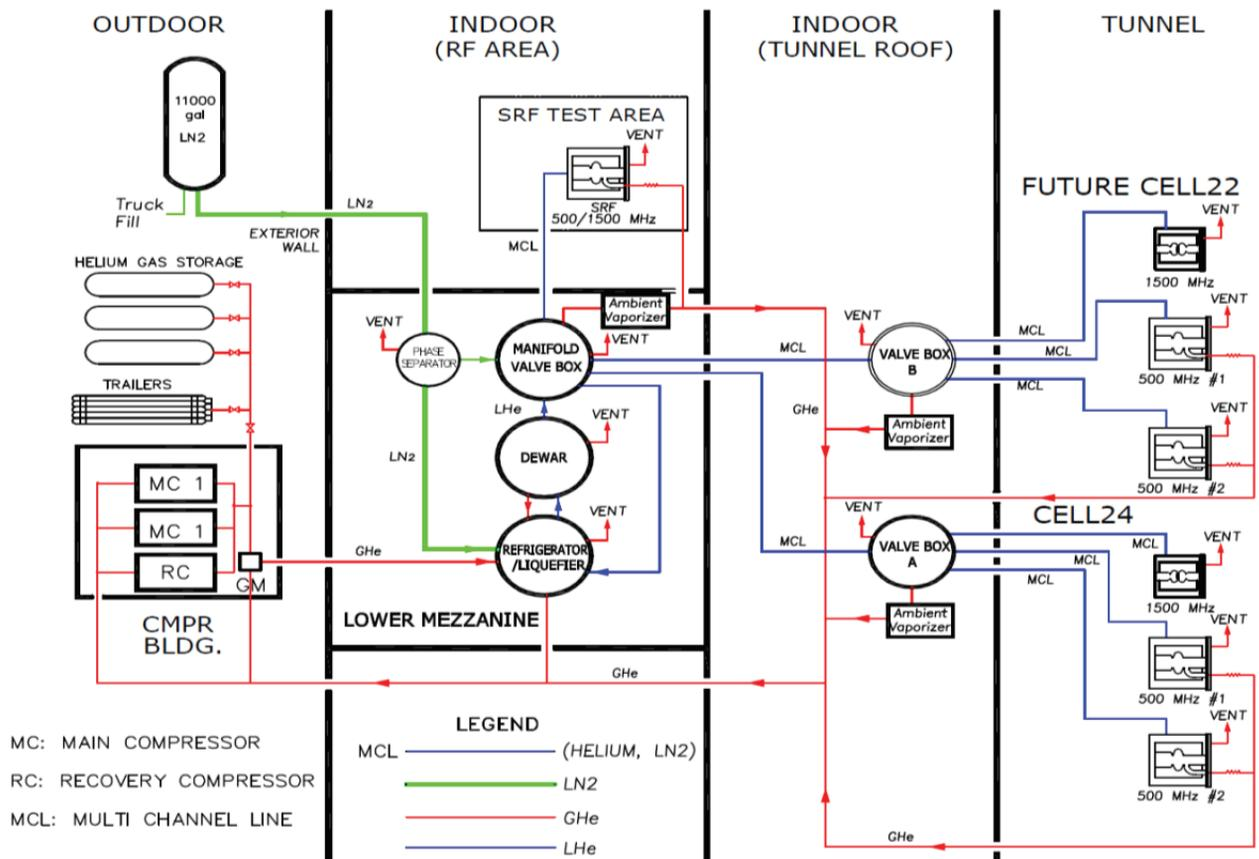
Figure 1: RF cryogenic plant diagram.
