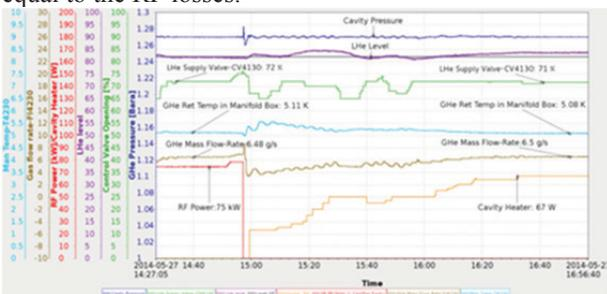
Figure 2: Calorimetric measurement of RF losses in the cavity.
