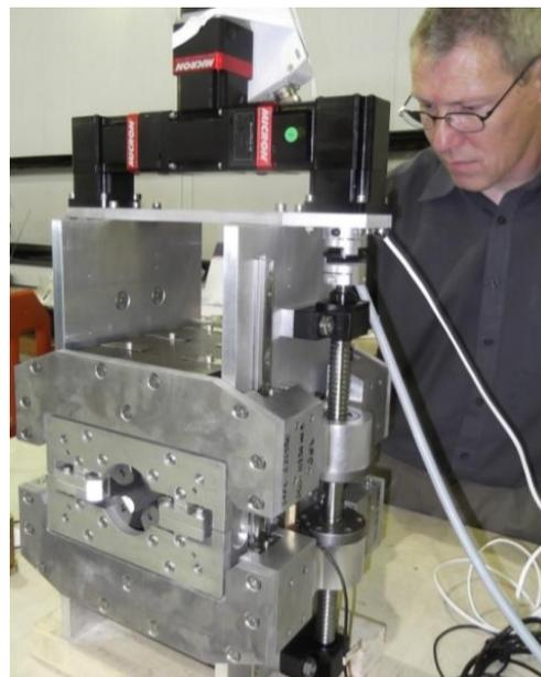
Figure 6: Permanent quadrupole with mechanical tuneability of the gradient between 15 and 60 T/m, developed for focusing of the CLIC drive beam [17].
