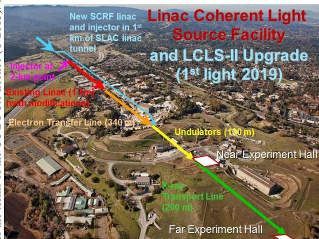
Figure 1: Schematic of the LCLS facility with the LCLS-II SCRf upgrade shown in blue.
