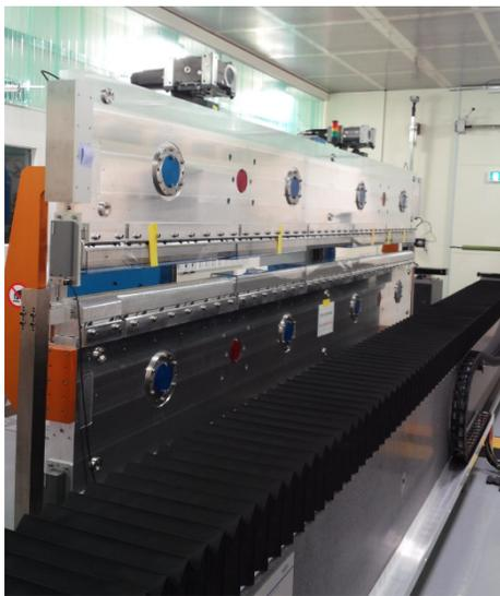
Figure 7: The first HX undulator under field measurement.
