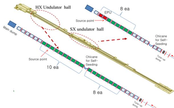
Figure 6: Undulator layout for HX1 and SX1. Green colour box represents an undulator to be installed.
