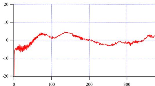
Figure 9: Optical phase error at the working gap of 9.5 mm. The vertical axis represents phase and the horizontal represents pole number.
