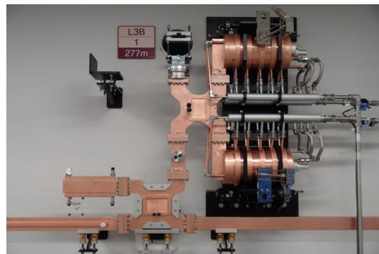
Figure 4: Picture of energy doubler and 3-dB power divider.
