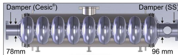
Figure 4: e-linac jacketed cavity with HOM dumper on each end.
