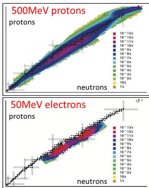
Figure 2: Yield production comparison between  $10 \mu\text{A}$ , 500 MeV protons on a  $25 \text{ g/cm}^2$  UCx target (top) and 10 mA, 50 MeV electrons on a Hg converter and  $15 \text{ g/cm}^2$  UCx target (bottom).
