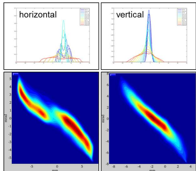
Figure 7: Beam profile as a function of solenoid strength (top) and relative tomography reconstructed transverse emittance (bottom).
