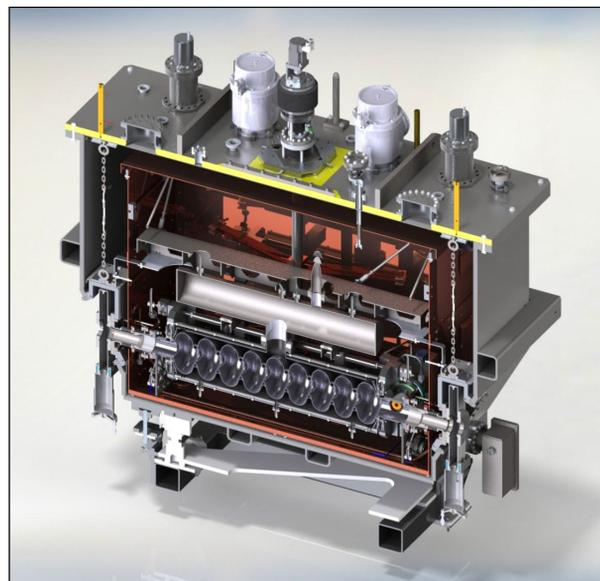
Figure 6: e-linac injector cryomodule rendering cross section.
