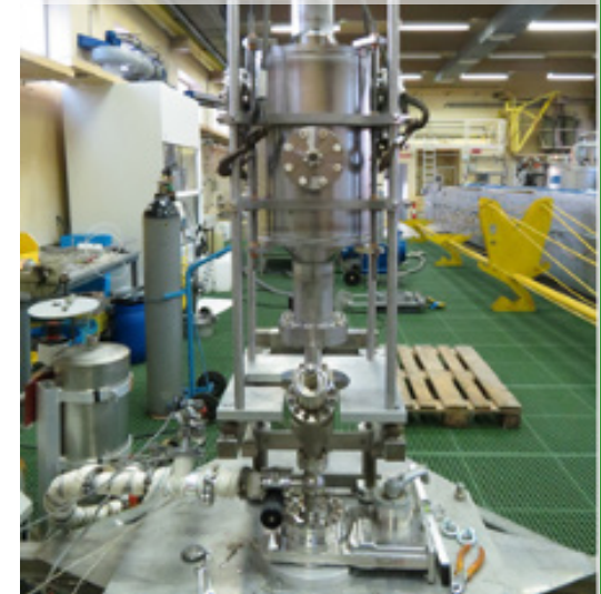
4-rod prepared for rinsing @ CERN
