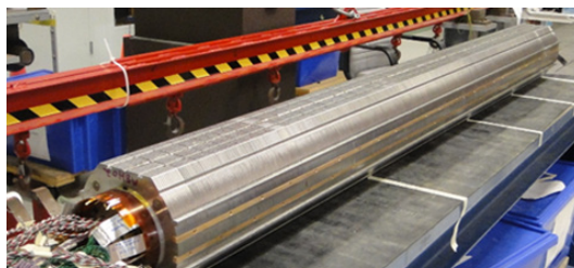
Collared coil assembly
