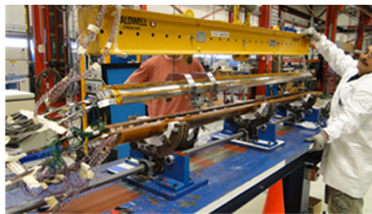
Collared coil assembly
