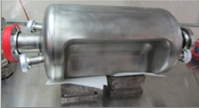
RF-Dipole Nb prototype [ODU-SLAC]
