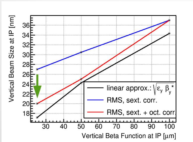
Decreased  $\beta_y^*$  causes the increase of  $\beta_y$  in the Final Focus region. In consequence the beam size is larger in the FF and more sensitive to beam line imperfections. It was checked that:
