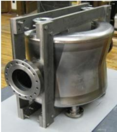
PoP DQW cavity with stiffening frame
