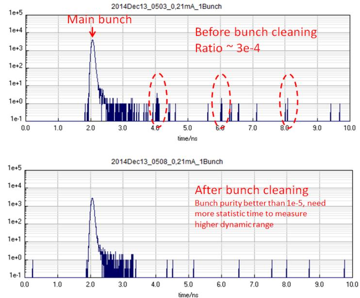
Single bunch purity measured using **Time Correlated Single Photon Counting** method
