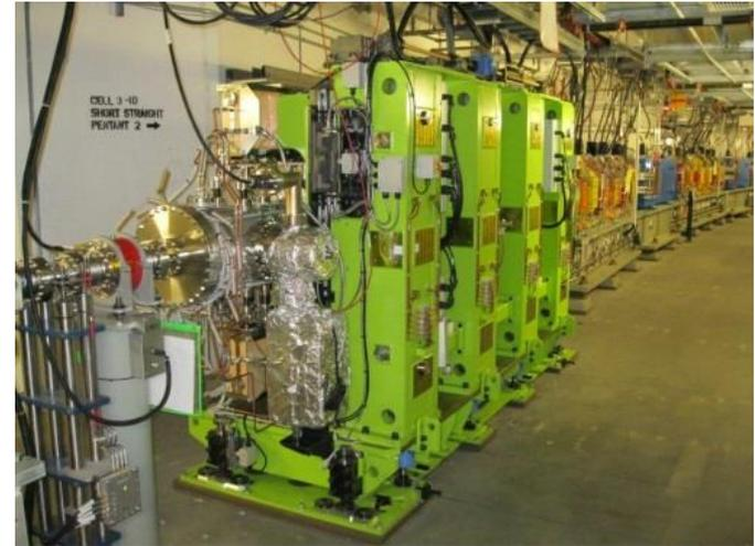
21 m of 1.85 tesla Damping wigglers
