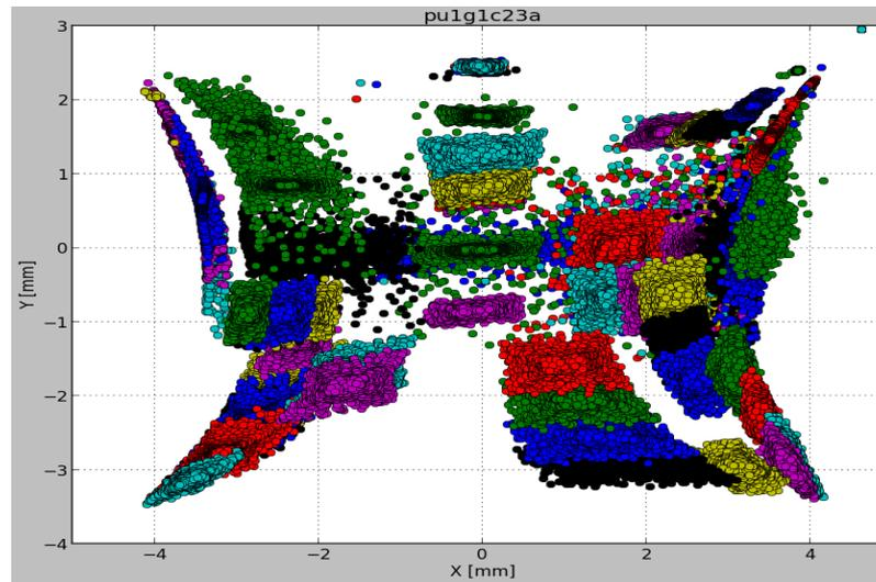
Automated 2-D aperture scan which uses a combination of DC and pulsed magnets
