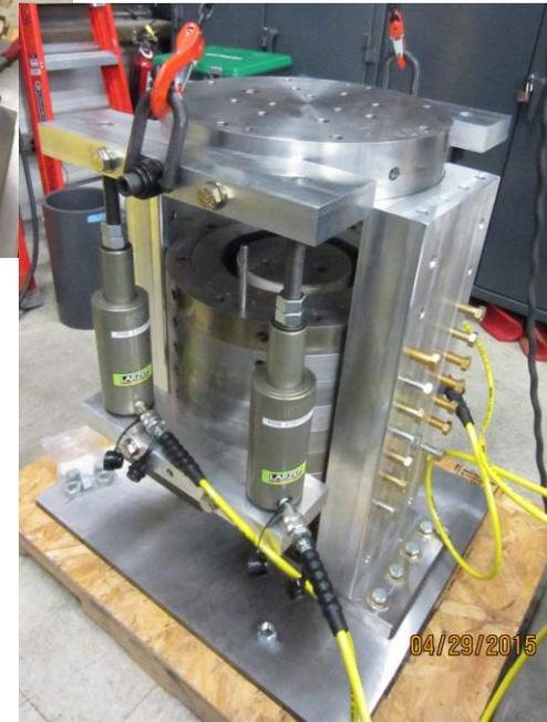
We have performed the assembly of the pump before the helical coiled tube was available. Four hydraulic cylinders control the ring motion.
