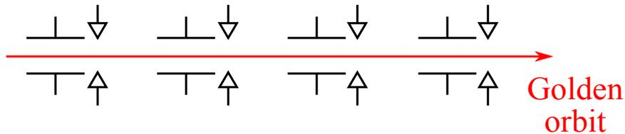
Orbit feedback steers beam onto golden orbit.
