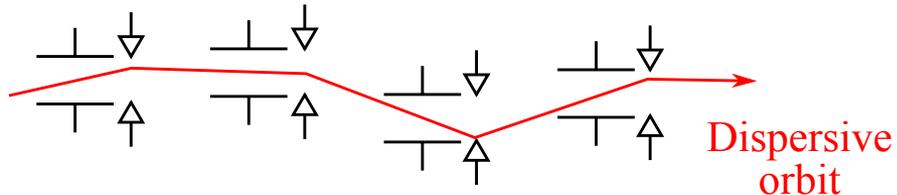
Orbit feedback steers beam onto dispersive orbit.
