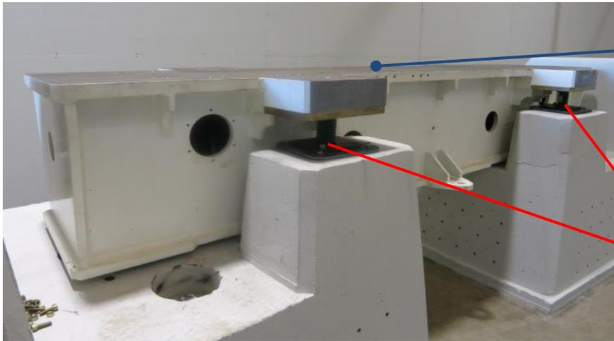
Accelerometers installed in 35 positions
