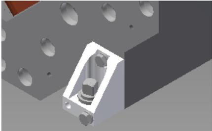
Goal: by definition assembly bellow  $\pm 20\mu\text{m}$  between adjacent magnets
