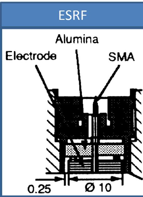
$r_{\text{button}} = 5 \text{ mm}$
