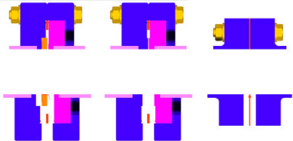
Fig. 4a CF Flange with RF bridge
