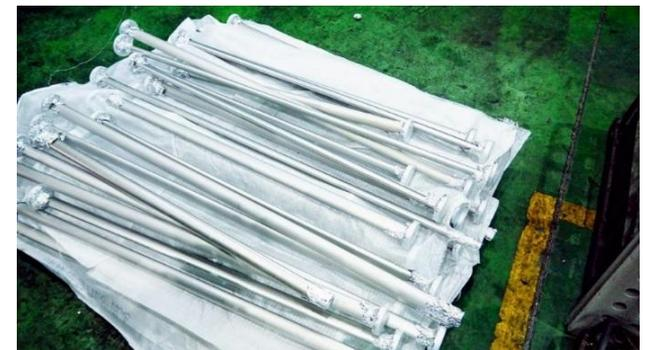
Shiny beam pipes after heat treatment
