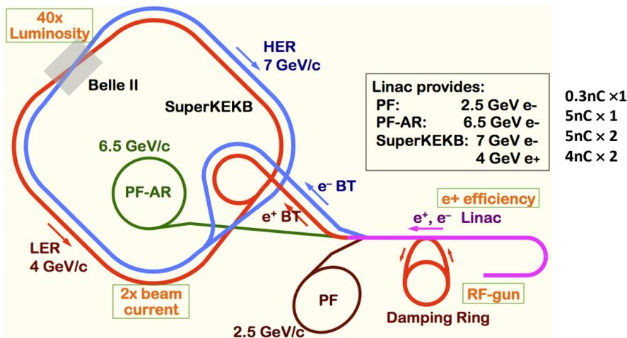
Beam modes are switched in pulse to pulse for 5-rings including Damping Ring (DR).
