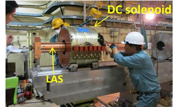
Solenoid field at e+ production target
