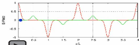
QTW is made by two standing waves with 90deg phase difference.
