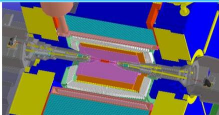
New superconducting final focus system
