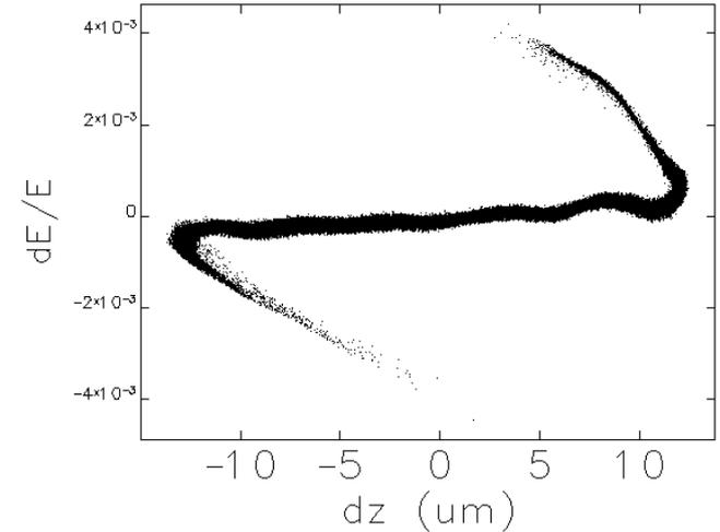
BFG of Undulator with 200 k particles
