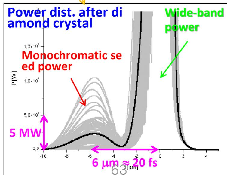
Self-seeding of 1-μm  $e^-$  pulse at 1.5 Å yields  $10^{-4}$  BW with low charge mode
