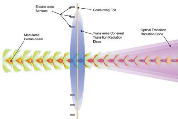
Figure 7: Schematic of the CTR and TCTR generation by a modulated particle bunch passing through a conduction foil.
