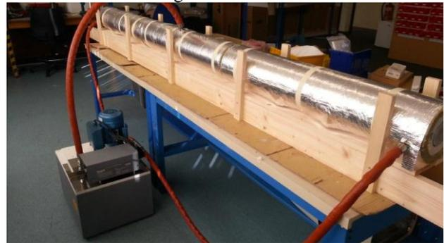
Figure 6: Prototype of a 3 m long Rubidium plasma source, courtesy of Grant Instruments Inc.
